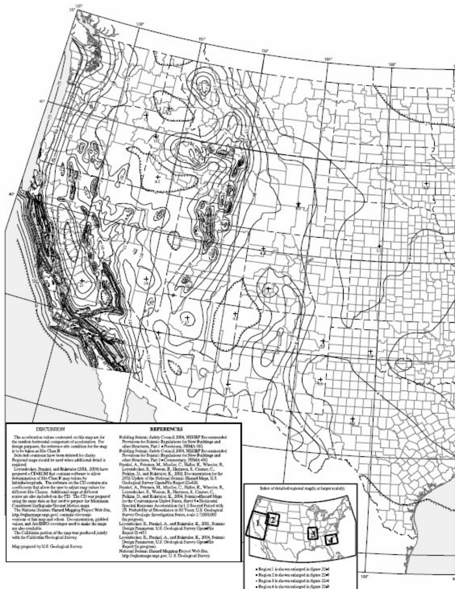
FIGURE 22-2 MAXIMUM CONSIDERED EARTHQUAKE GROUND MOTION FOR THE CONTERMINOUS UNITED STATES OF 1.0 SEC SPECTRAL RESPONSE ACCELERATION (5% OF CRITICAL DAMPING), SITE CLASS B
