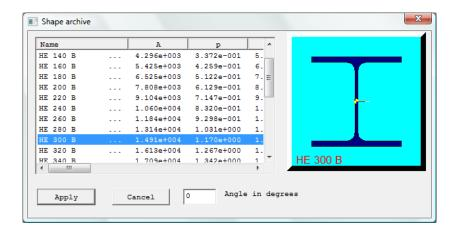
HEB300 is now the current section. Click the "Assign current!" button on member 1 row to assign current shape to member 1 (the master).
