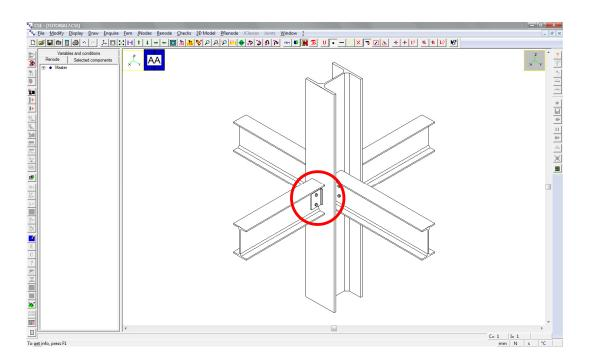
In this example we just modified the thickness of a plate, but also other components and operations can be changed. For example:
