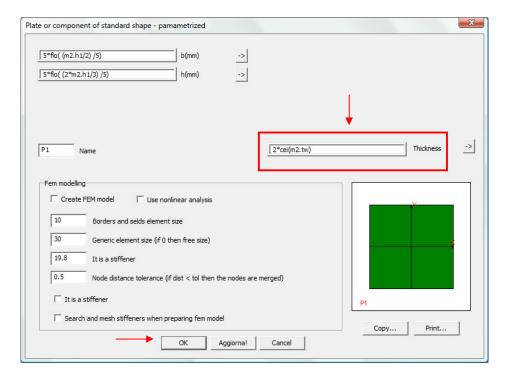
Renode construction is automatically completed. Now P1 is thicker and other components are coherent with this modification (for example, weld layout connecting P1 to the master).
