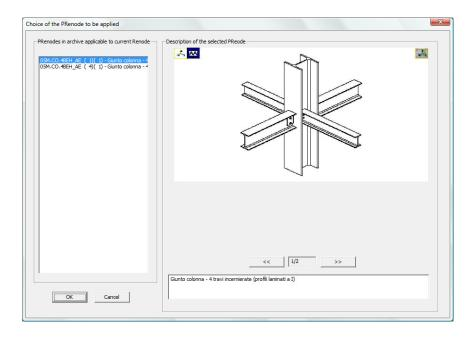
N.B. now there are two possible applications of the same prenode: they have the same name, but one ends with (1)(1) and the other one with (4)(1). This happens because during the first application of the prenode slave members were renumbered to fit the order saved in the prenode. Now, with the new renumbering, there are to possible applications of the same prenode. Click OK to apply the first one.
