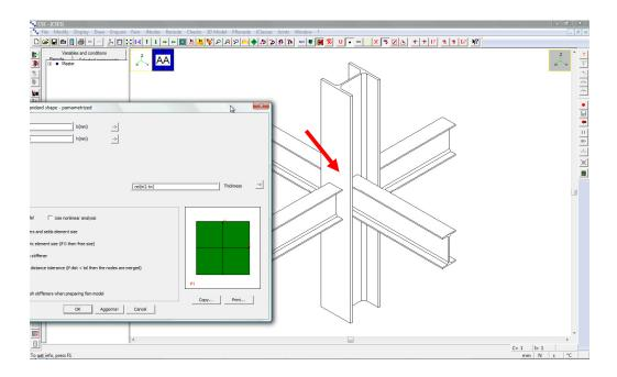
In the dialog box for P1 plate definition, modify for example the thickness of the plate. In order to clearly understand what happens, define a thickness that is the double of previous one: current thickness is cei(m2.tw), it means equal to the tickness of member 2 web rounded up to the nearest integer. Type "2\*" in order to get 2\*cei(m2.tw), twice the original plate tickness, then press OK.
