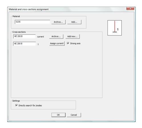
It is possible to apply a rotation of 90° to the member removing the tick from "Strong axis" box. In some nodes, not in this case, it is possible to define hinges for the slaves with proper tick boxes.
