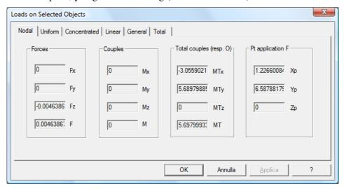
This is the resultant of all the nodal forces applied to all the selected nodes. Notice that the resultant is quite low. Also notice that the point of application of resultant is near, i.e. not at an infinite point. This means that not only the force resultant is low, but also the moment.
