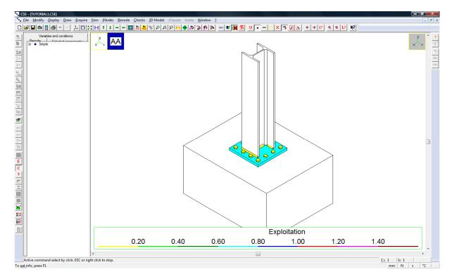
This is the element in traction (0.1 times the elastic force). Note that the constraint block is not loaded by any pressure. By pressing the button in the main toolbar you move to the following combinations. You notice it in the status bar at the bottom of the CSE window.
