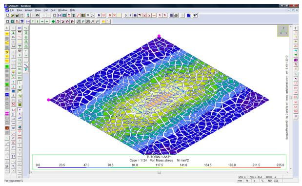
The plate is OK in this load case 1 (column pulled by 0.1 times its elastic limit). Switch to combi 7 by using the same button you already know in the main bar. You see what follows:
