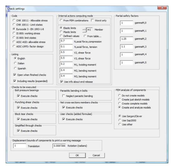
Leave all the remaining data as default suggests. Just ask "Create and analyse models" in order to get the fem model of the plate to be solved. Choose Sargon/Clever, i.e. the embedded solver, as solving tool.
