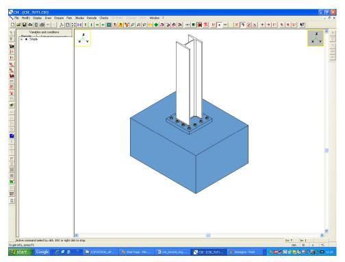
However, since the bolt length has changed (due to the increase in plate thickness) we have to inform the program by just re-editing and saving the bolt layout. You can notice this thing in two ways.
