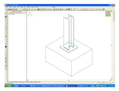
Bolts will drill into that face to connect the plate to the constraint block. As soon as you click left choosing the top face you get into this dialog:
