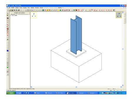
Now let's add the bolts joining the base plate to the constraint block. Unselect all objects by pressing
