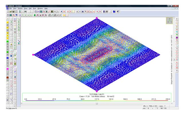
Although there is an area where the Von Mises stress is higher than 235MPa, we would probably accept this plate element, as the plasticization occurs in a limited region under the column web.
