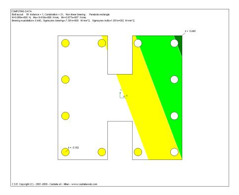
As we can see from these pictures, the no-tension compressive field over the bearing surface is correctly computed. The bolts in tension are drawn in colour, the compressed bolts do not react (this was a choice of ours in the bolt layout properties, see the "Compressed bolts" check-box).
