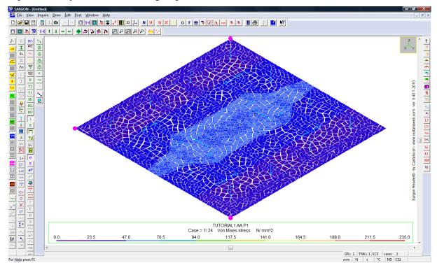
Now look at the next 5 combinations, the stresses are always low. So it is the compression in the column to produce the high stress. See now load case 7: this is the compression. You see that the stress map is as follows (we have removed the loads by using View-Objects command, and removed the tick from "Loads", and set the plate elements shrink to 1 by pressing button in the main bar and setting 1 as shrink):
