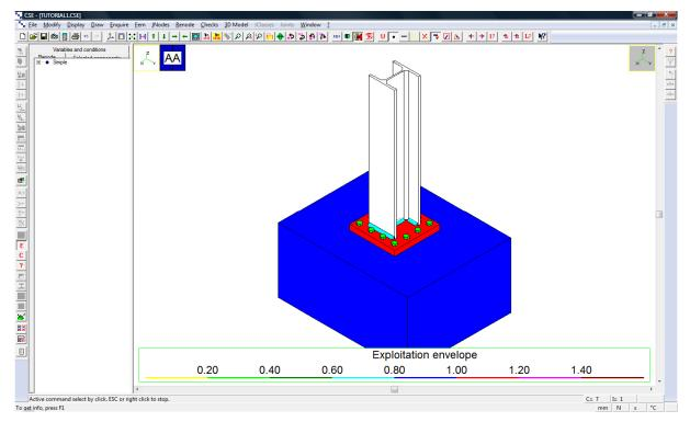
The weld is now exploited at a lower level, and once more checked, while the plate is still not (1-1.2 range, a lower range than before, but still un-checked). However we would like to have a look at the fem result to decide if the plate can be accepted or not. Select the plate by clicking over it and press the button in the left toolbar. Get into Sargon Reader and zoom in to have a look at the model.
