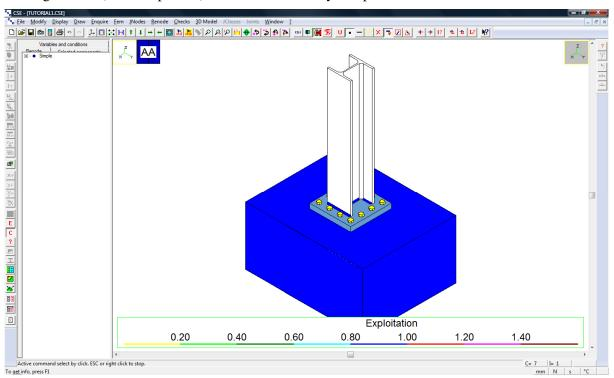
Just press the button in the left toolbar. This starts Sargon Reader to have a look at the FEM model created and solved for the base plate.
