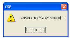
This is the "logic" of the real node. You go from member "m1" to the constraint block passing through W1, P1, and B1.
