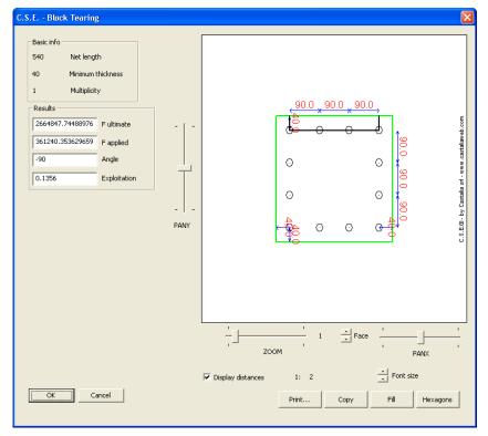
Note that the elastic shear has been computed as 722480N ( $2x200mmx15mmx235MPa/\sqrt{3}=814062N$ , 10% higher, Eurocode 3 uses a slightly different formula to compute limit shear, as shear 3 uses part of the flange area), and that 0.5x722840=361240N. The block shear check assume - on the safe side - that all bolts pull in vertical direction creating the shear+tensile rupture shown in the picture. This is the worst possible path. Exploitation is quite low.
