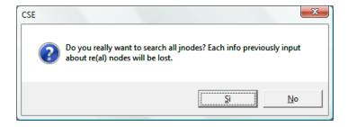
As no real nodes info has been defined you won't lose anything. Jnode search is usually done once for all in a model. Before beginning to add RENODES, you will check that the JNODES found are correct. This depends also on how the fem model has been prepared.
