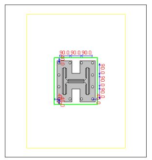
As you will notice clicking over the Face arrows, the face chosen as bearing object will be shown yellow. We have defined both the bearing surface and the bearing object for the bolt layout. Please note that this is needed only when using bolt layouts that use the bearing surface concept.
