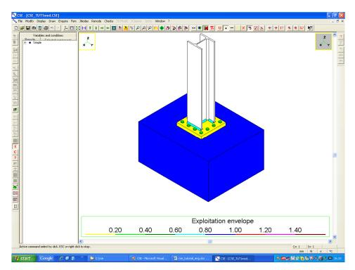
Every component is checked. The plate has been previously studied via fem Let's have a look at the constraint block checks. Here what matters is the pressure over the block. Exit from the "E" command and select the bolts by clicking over them. Now press the button in the left toolbar.
