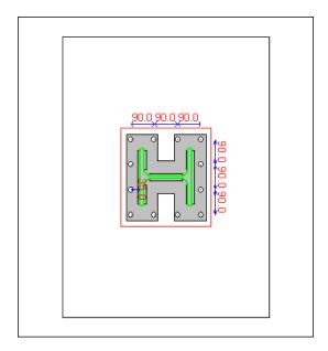
So we will use this surface as bearing surface for the bolt layout. The bearing surface will only react in compression.
