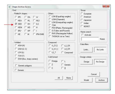
Select HEB check box and then "Archive" to filter HEB kind among all the available cross-sections. Then choose the section HEB200 by selecting the appropriate row, and press the "Apply" button.
