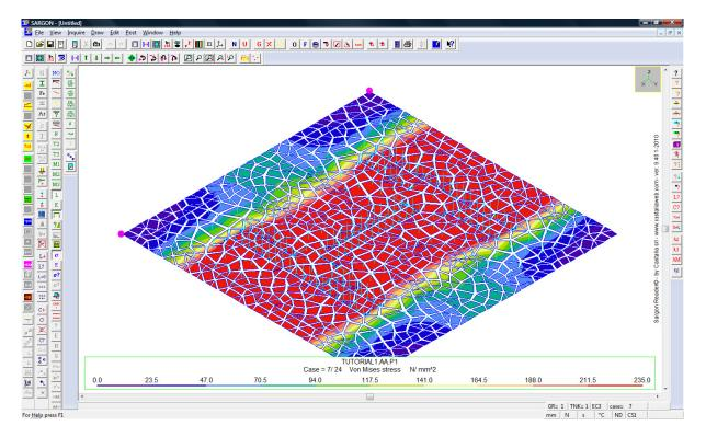
We will then change the plate to a higher thickness and also change the weld that highly exploited (0.973 < 1).
