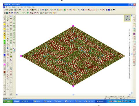
The model is more refined. Now choose the stress button ( ) in the left toolbar, as already explained. Choose Remove interelement jumps and press OK. You see the Von Mises stress map in
