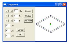
This point will be the insertion point of the object. Now press OK and click the bottom face center of the member. The plate will be placed so that its insertion point will match the point chosen. Orientation will be the same.
