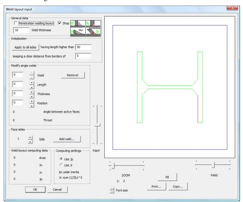
Choose the weld thickness, for instance 10 (mm, as we are using default units).
