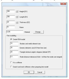
N.B. in latest versions, default values have been changed: angle is  $18.9^{\circ}$  and tolerance is 0.5 mm.
