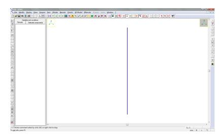
Members (only one in this case) appear in the jnode view. In general, structural members do not coincide with finite elements: for example, a single member can be divided into 2, 3 or n finite elements.
