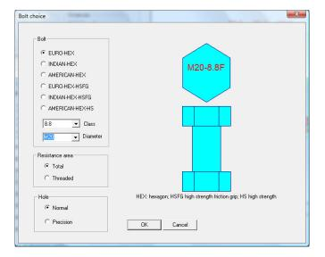
Keeping EURO-HEX selected, choose the steel grade 8.8 and the bolt diameter M20 (mm). Then leave the default Total resistance area, and Normal hole. Press OK. You are back in the previous dialog, but now the bolt is M20-8.8.
