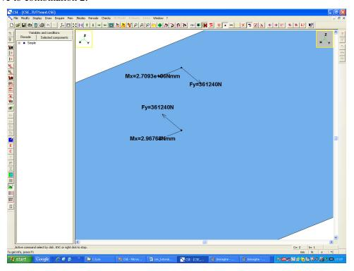
The shear 2 at the base of the column (we have seen it is equal to 361,240N), when moved at the second weld extreme gives rise to a moment equal to 2,709,300Nmm, that is 361,240x7.5mm, which is half the actual weld thickness). In CSE every parasitic moment is kept into account.
