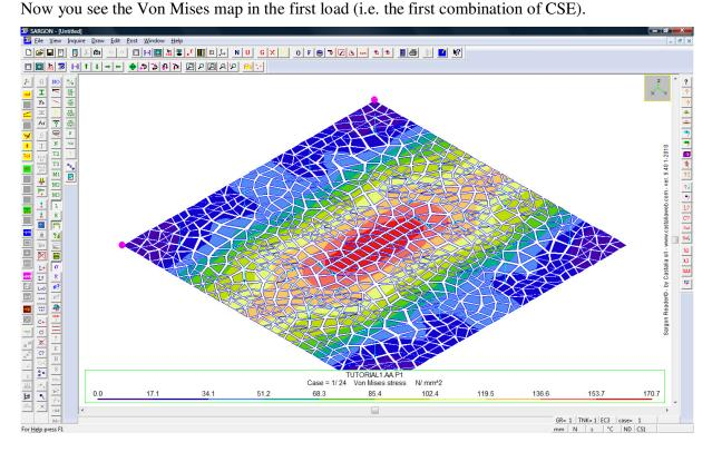
To better understand the stress levels, set as maximum stress the yield stress in the stress scale. Execute Post-Legend command, remove the tick from Automatic and set as maximum 235 ([N/mmq] as you are using default units).
