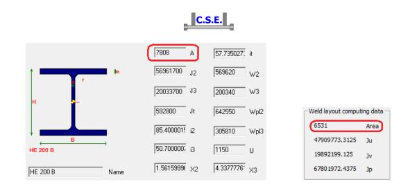
Area of HEB200 = 7808 mm<sup>2</sup> Weld layout total area = 6531 mm<sup>2</sup>
