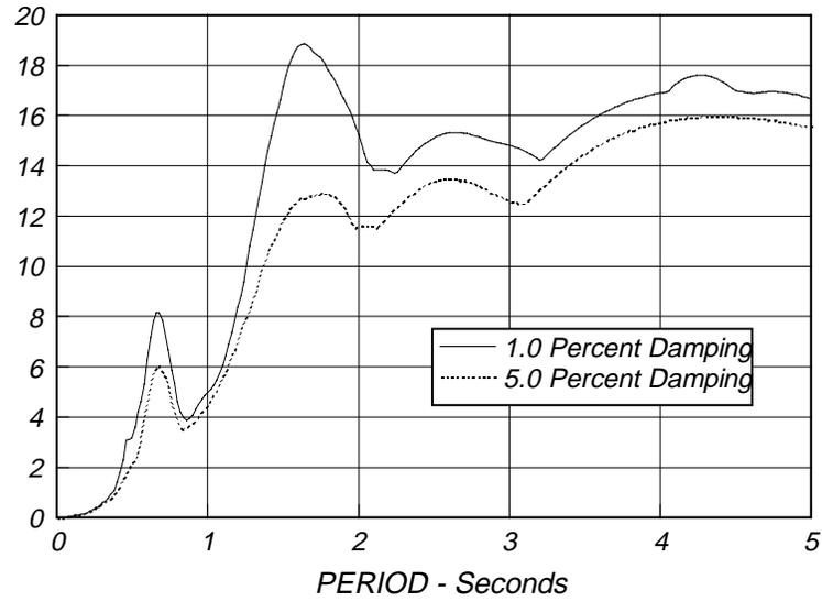
**Figure 15.2a. Relative Displacement Spectrum  $y(\omega)_{MAX}$  - Inches**
