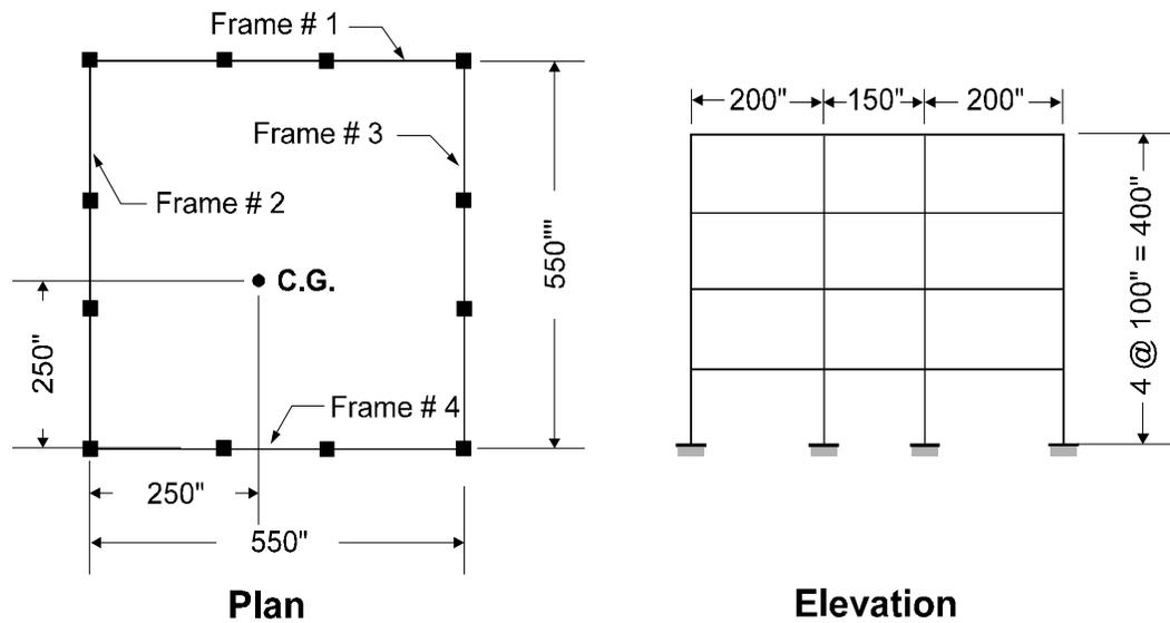
*Figure 15.3. A Simple Three Dimensional Building Example*
