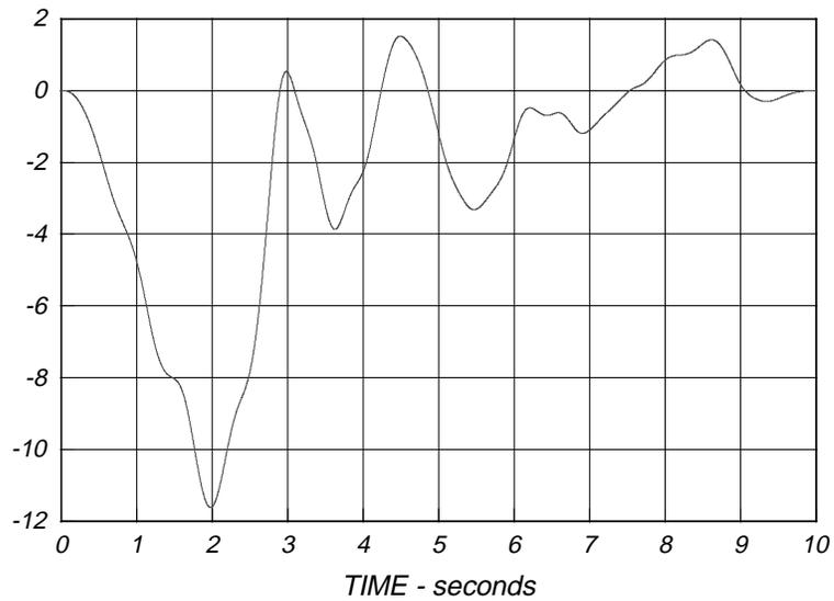
**Figure 15.1b. Typical Earthquake Ground Displacements - Inches**
