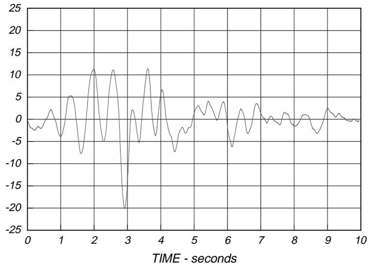
**Figure 15.1a. Typical Earthquake Ground Acceleration - Percent of Gravity**
