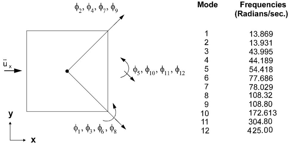
**Figure 15.4** Frequencies and Approximate Directions of Mode Shapes
